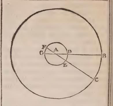
Let the line GAB, represent a ballance or leaver, the weight being supposed at the point G, the sulciment at A, and the power sustaining the weight at B. Suppose the point G, unto which the weight is fastned, to be elevated unto F, and the opposite point B, to be depressed unto C; 'tis evident that the arch FG, or (which is all one) DE, doth shew the space of the weight, and the arch BC, the motion of the power. Now both
